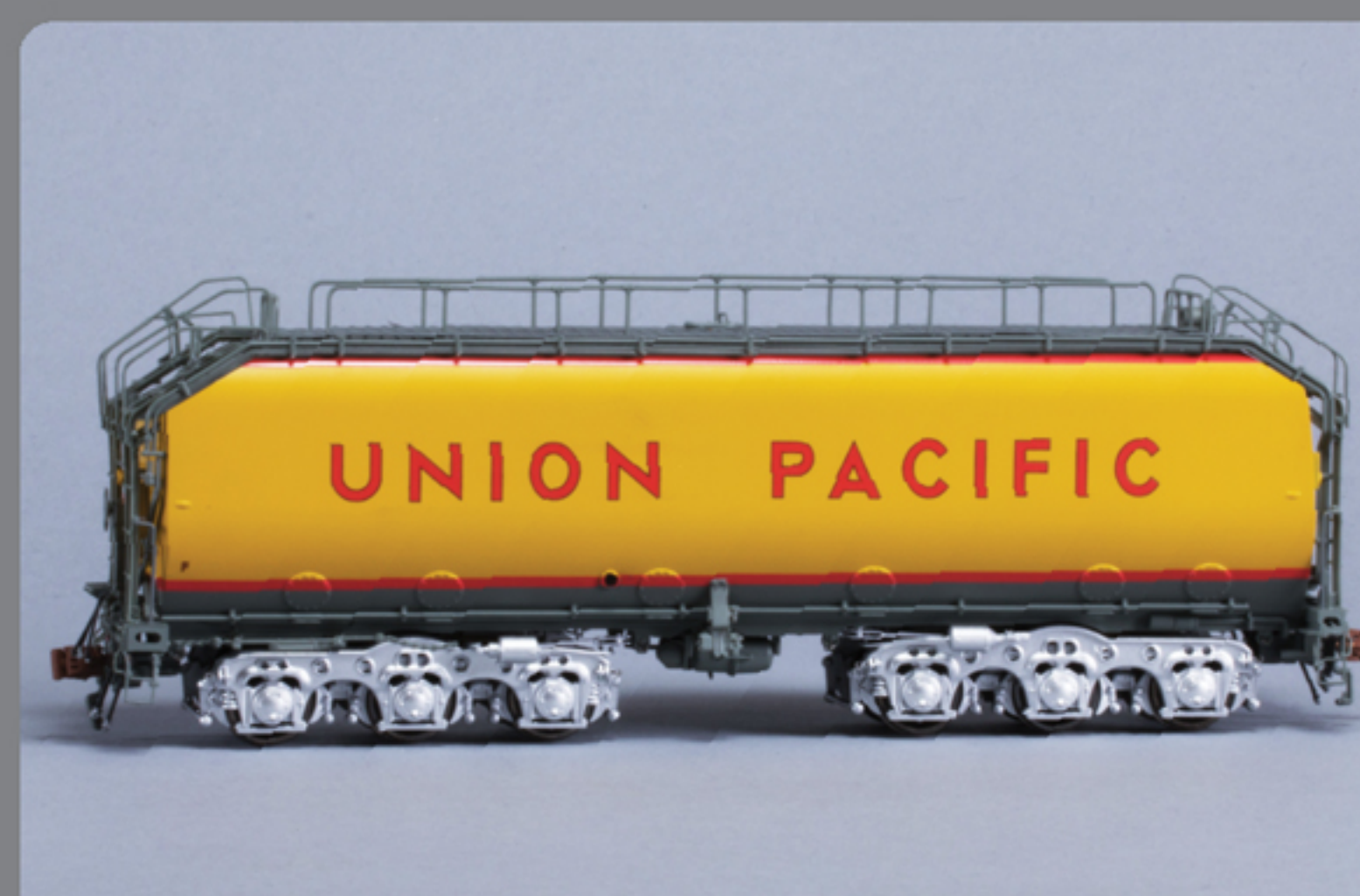
Smooth-sided construction of the 24C tender and its "Commonwealth" 6-wheel trucks.
