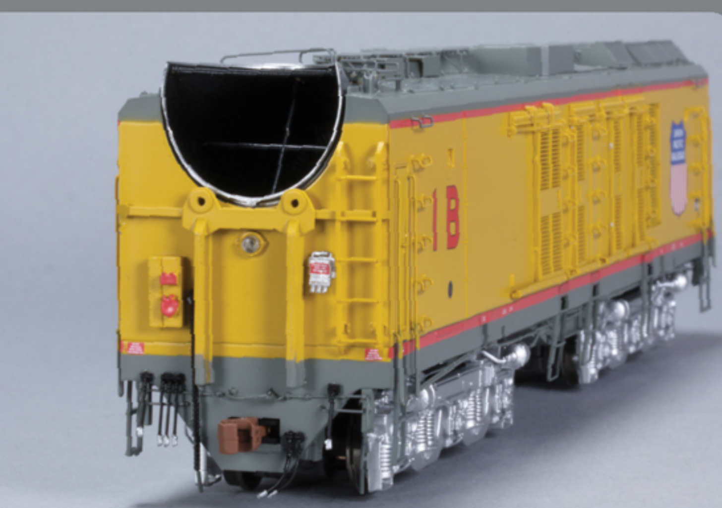
The rear of GTEL B-Unit #1B, shows off its as-built rooftop air intake system, operating back-up light, and exhaust housing.
