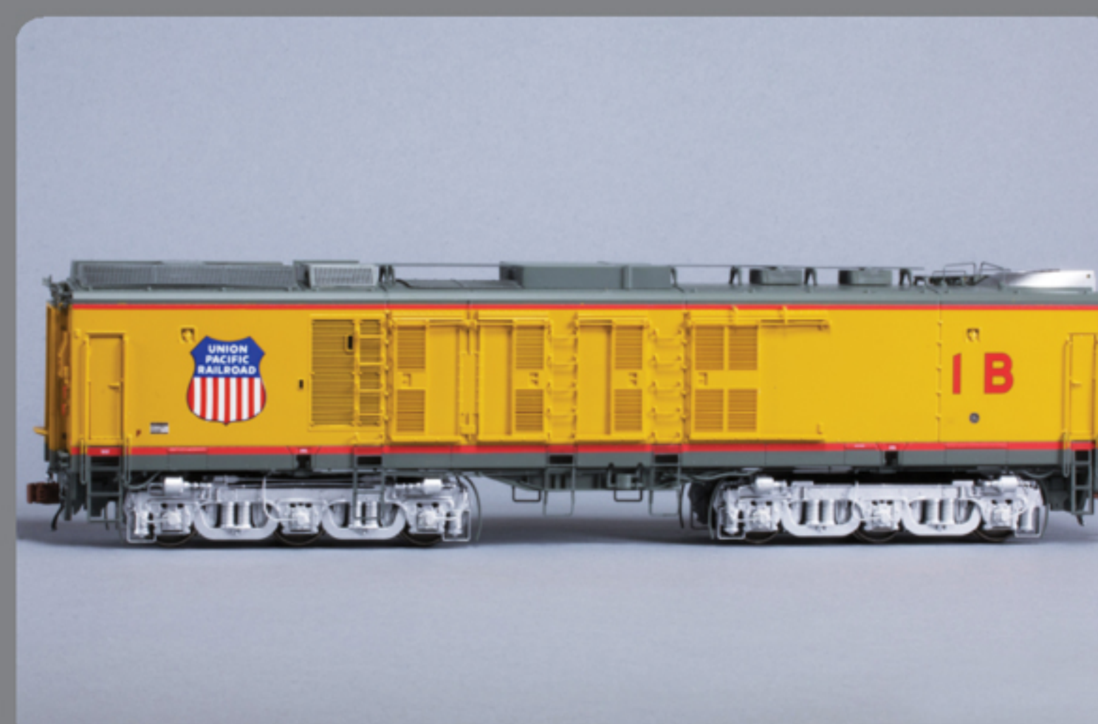
Profile of UP GTEL B-Unit #1B with its as-built air intake box on the roof and early "H-I" dynamic brake housings.
