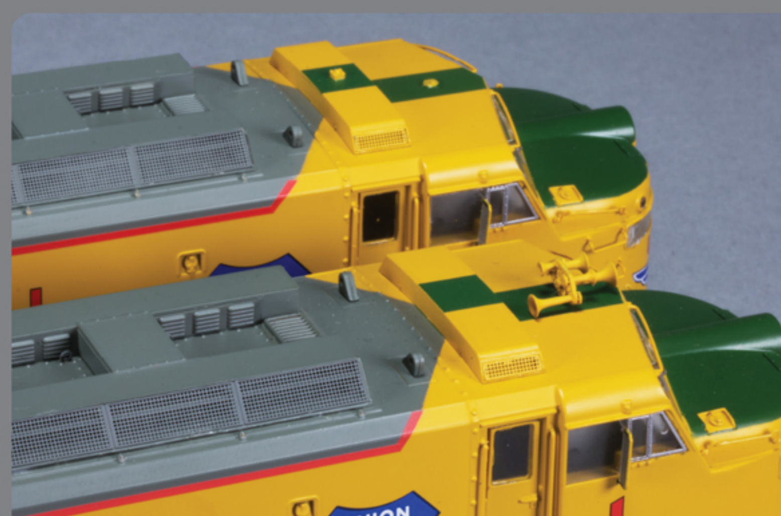
Rooftop details on the GTEL A-Unit cab roof include cab heater box, lift lugs, windshield grab irons, and more.
