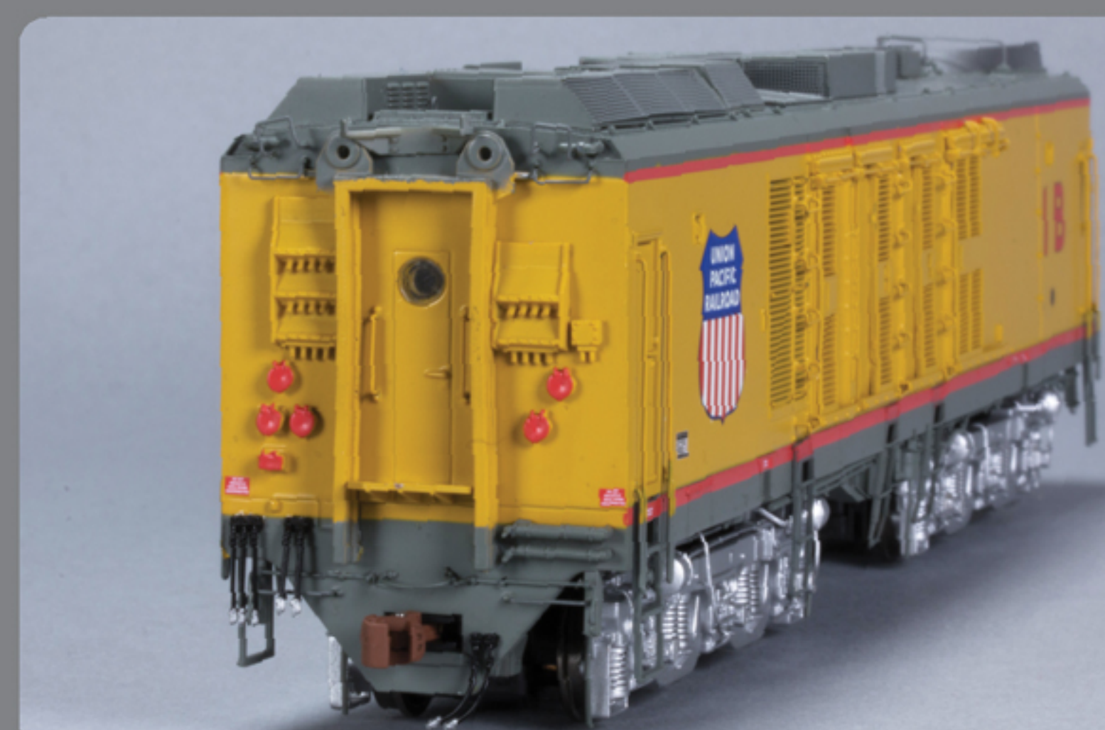
The front of GTEL B-Unit #1B. It has early "H-I" dynamic brake configuration, and electrical connectors.
