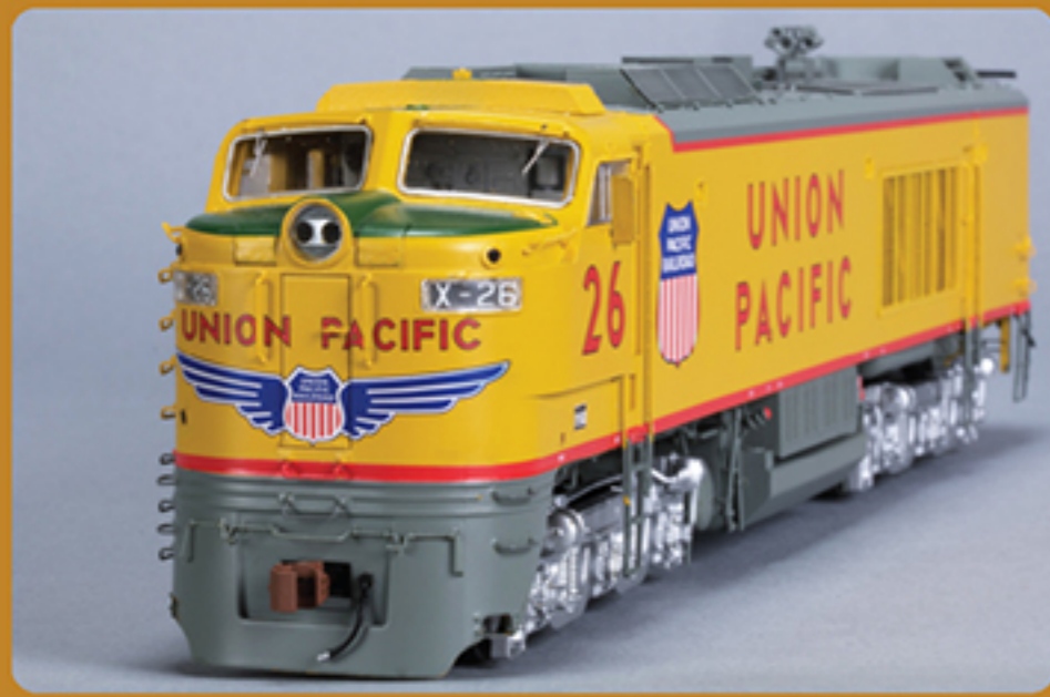
Late-era details on UP #26, including relocated horn, and grab iron ladder on right side of nose.
