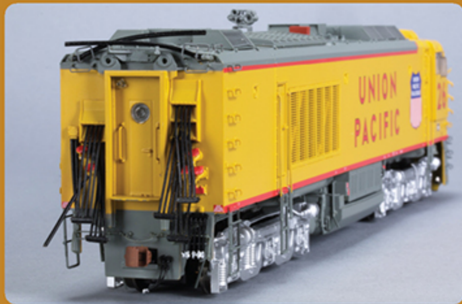
Rear of GTEL A-Unit 26B showing the flexible rubber electrical bus cables and MU cables for installation between the A and B-unit
