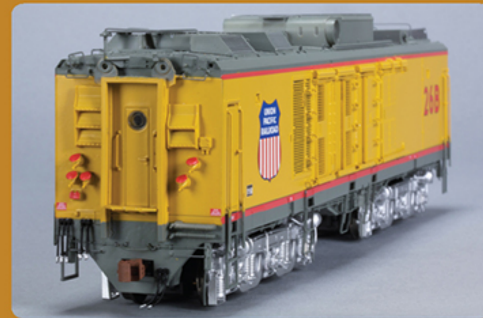
MU connection, lift lugs, and "I-I" details on the front end of the GTEL B-Unit #26B.
