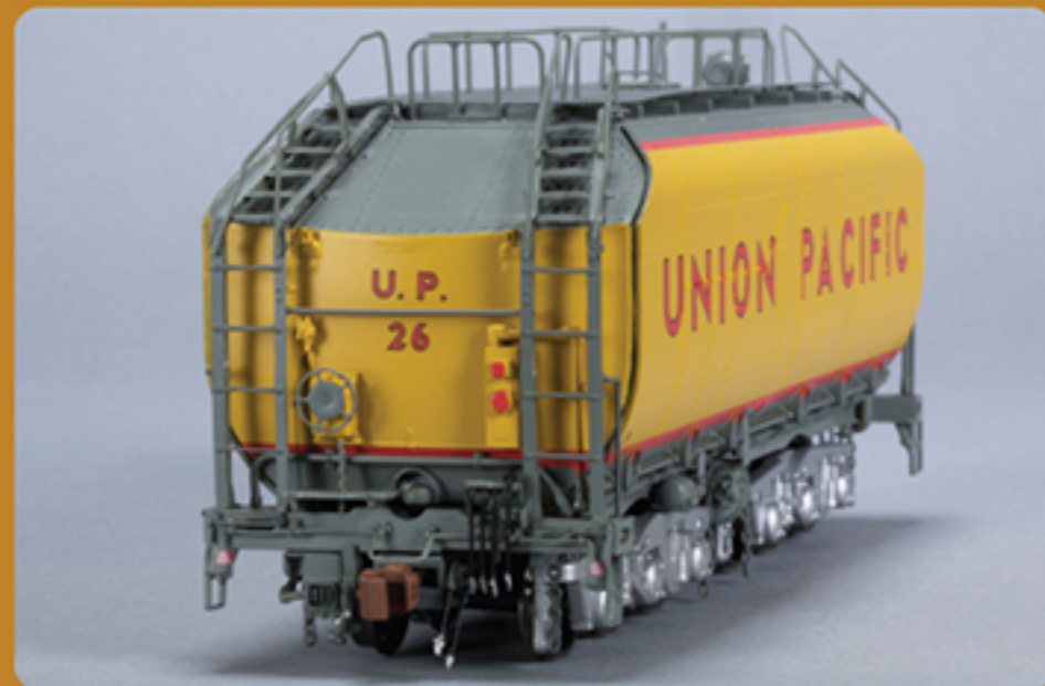
Stunning detail on the front of the 23C tender, including electrical connections, handbrake, and fine ladders and steps.
