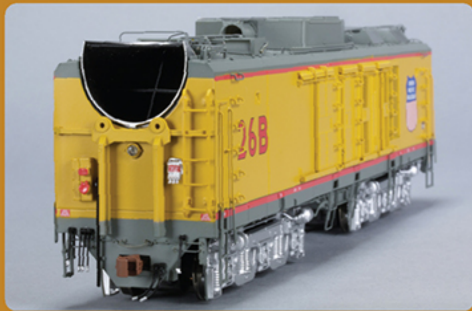
Rear of GTEL B-Unit #26B, showing the rear of the rooftop "Dynavane" air intake system, operating back-up light, and exhaust housing.
