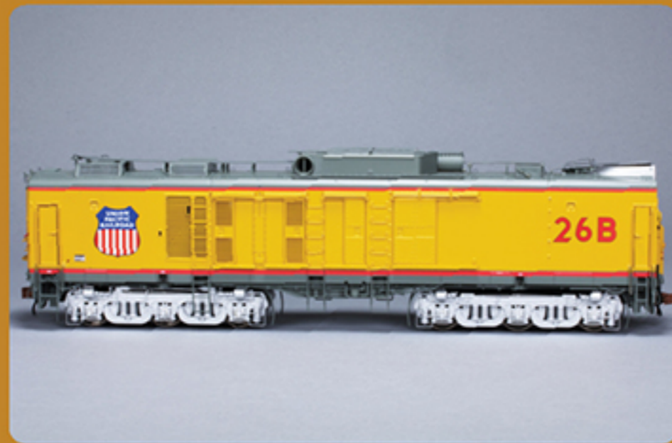
GTEL B-unit #26B showing its retrofitted "Dynavane" air intake system, "I-I" dynamic brake housings, and intricate grab iron and step details.
