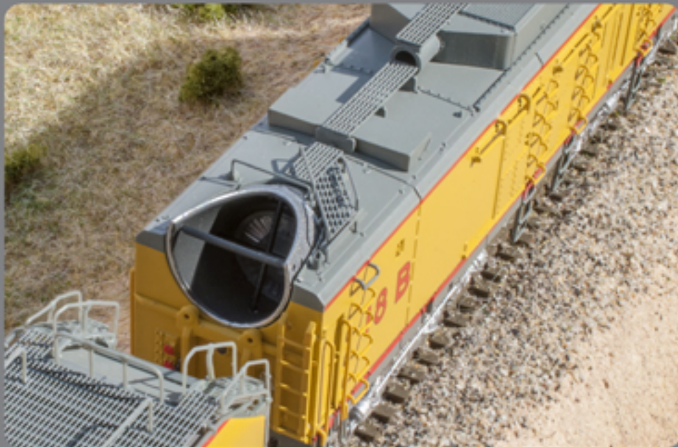
Photo-etched B unit walkway. Wireform grabirons and exhaust detail.
