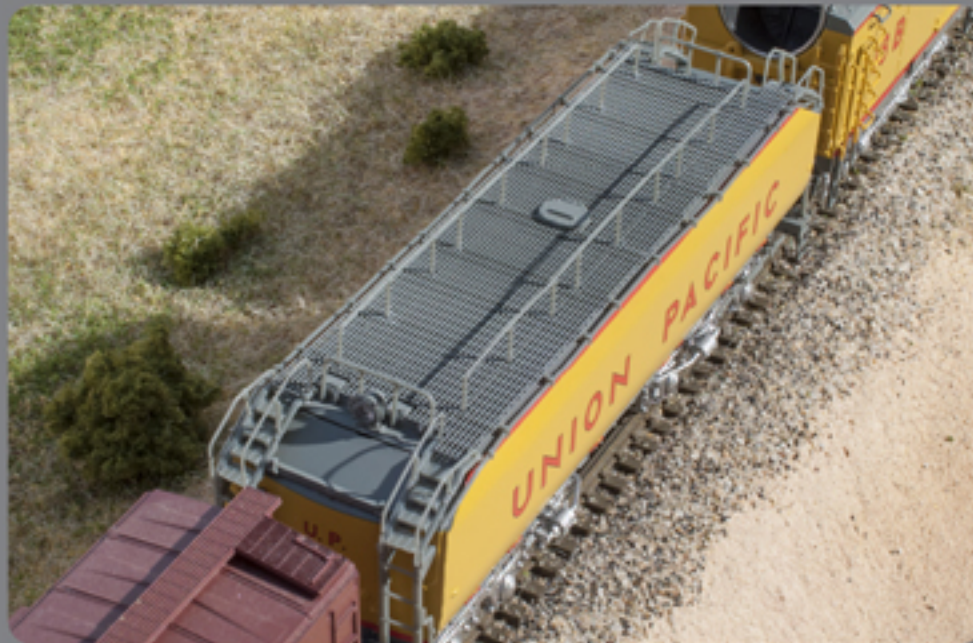
Photo-etched tender walkway. Separate tender deck handrails.
