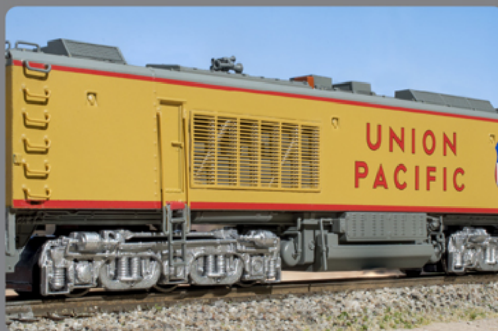
Photo-etched see through side grille detail on A unit.
