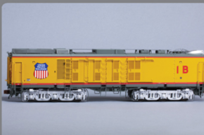
Profile of UP GTEL B-Unit #18 with its as-built air intake box on the roof and early "H-I" dynamic brake housings.
