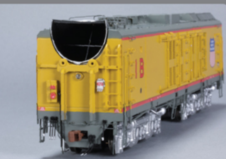
The rear of GTEL B-Unit #18, shows off its as-built rooftop air intake system, operating back-up light, and exhaust housing.
