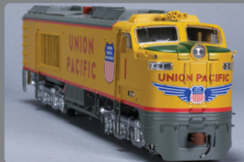
As-delivered details on UP #1, including cab-mounted horn, and no grab iron ladder on right side of nose.
