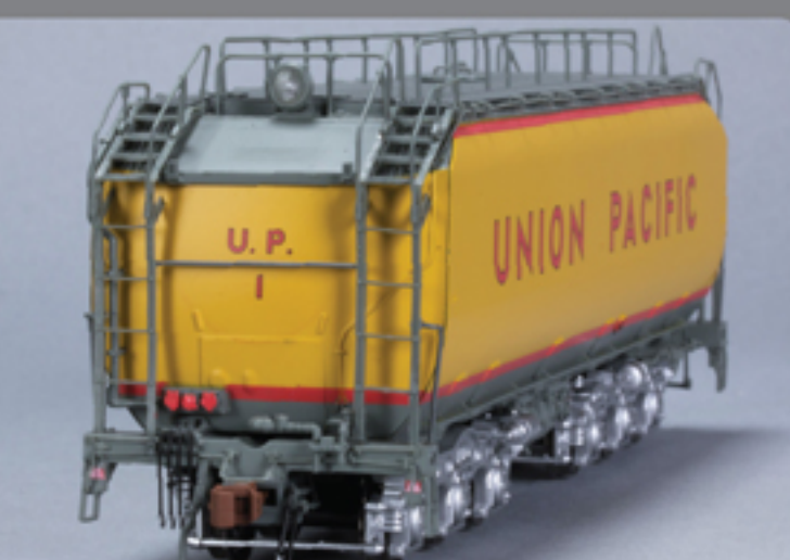
Finely detailed 24C insulated tender, featuring fine plumbing and electrical connection details on the front end.
