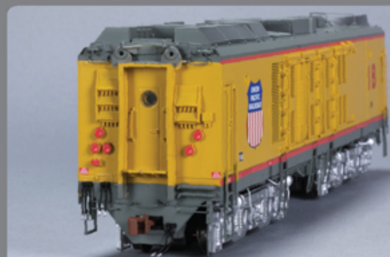
The front of GTEL B-Unit #18. It has early "H-I" dynamic brake configuration, and electrical connectors.
