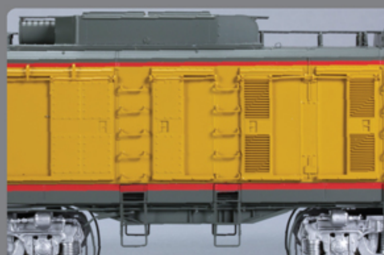
Sharply detailed access door and grab iron details on the sides of the GTEL B-Unit.
