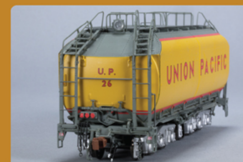
Detailed rear end of the 23C tender, showing its operating back-up light, and separately applied plumbing details.
